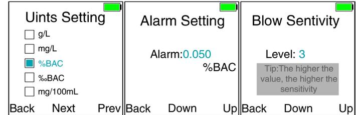
In the “params”, you can select different units, alarm threshold, blow sensitivity adjustment, with the number starting from 1 to 5, which corresponds to low to high sensitivity.
